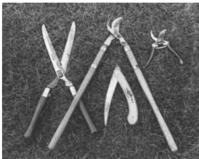
Figure 1.—Tools used in pruning include (left to right) hedge shears, loppers, pruning saw, and hand pruners.
