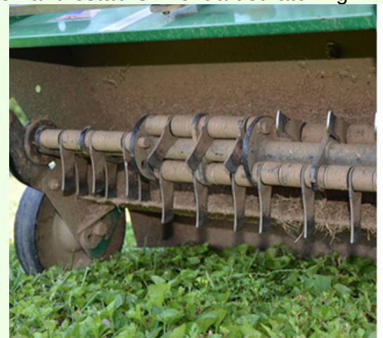
The underside of a dethatching machine showing the sling blades that remove thatch and create small furrows in the soil. Source: Gregg Munshaw, University of Kentucky Plant and Soil Sciences
